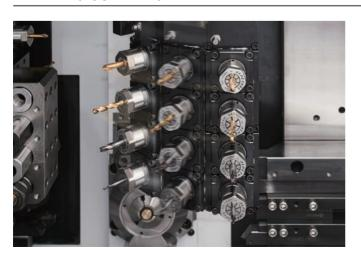
4 x double ended spindles, 0-135 deg, usable for both main and sub spindles.
