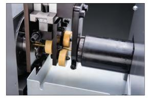
Cincom's unique bar and spindle stabilizing mechanism aligns precisely the bar's center of rotation with the center of the spindle. Forces are evenly distributed, protecting the spindle from excessive wear.
