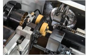
Oil/Roller Support System: As the bar rotates, it becomes hydrostatically supported in a bath of oil and perfectly centered in the guide channels. Even with full-length, 13' bars, the lathe can operate noisefree and vibration-free at speeds to 15,000 rpm.
