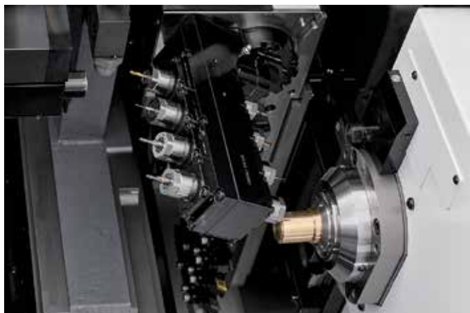
B-axis rotary tools on the gang tool post
